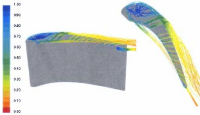
Fig. 10 Predicted path lines for the 0.58% coolant flow at the small tip gap
